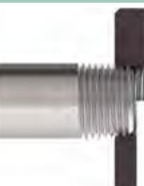
The GO/NOT GO thread plug gauge cannot be screwed in above the maximum step. The GO/NOT GO thread ring gauge cannot be screwed on until the maximum step is reached. The workpiece thread is oversized.
