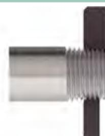
The GO/NOT GO thread plug gauge cannot be screwed in until the minimum step is reached. The GO/NOT GO thread ring gauge cannot be screwed on above the minimum step. The workpiece thread is undersized.
