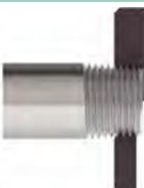
The thread gauge can be screwed (in or on) between the minimum and maximum step of the thread gauge. The workpiece thread is in tolerance.
