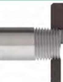
Thread gauge can be screwed (in or on) until the maximum step of the thread gauge is reached. The workpiece thread is up to the maximum size.
