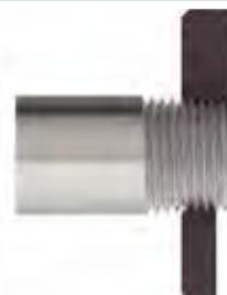
The thread gauge can be screwed (in or on) until the minimum step of thread gauge is reached. The workpiece thread is up to the minimum size.
