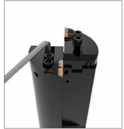
Step 3 Tighten the mounting screws on the cartridge to 11-14 ft-lbf (15-19 N-m).
