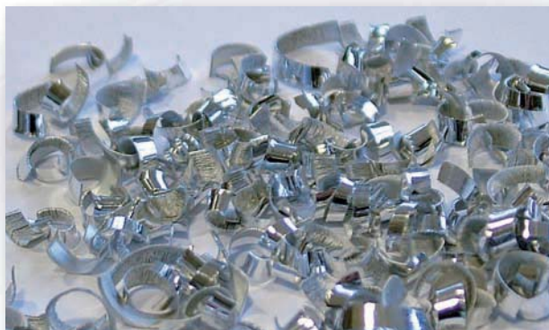
With 3D-chip breaker: Breakage chips
