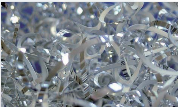
Without 3D-chip breaker: Flow chips
