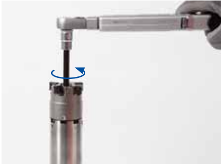
1. Loosen the milling cutter clamping screw, for example by using the torque wrench.
