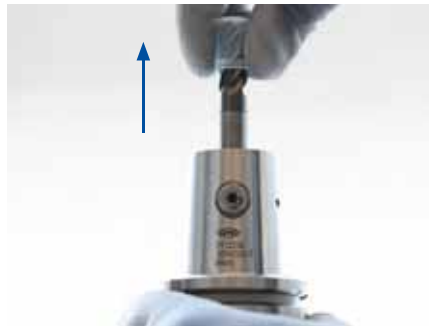
2. Remove the tool from the side lock chuck's location bore.
