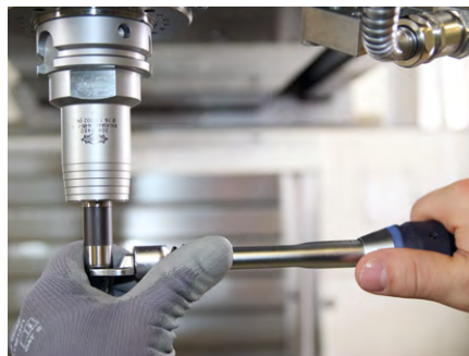
5. Note: Place your free hand on the replaceable milling head to be able to make delicate adjustments. This allows the tightening torque to be set more precisely.
