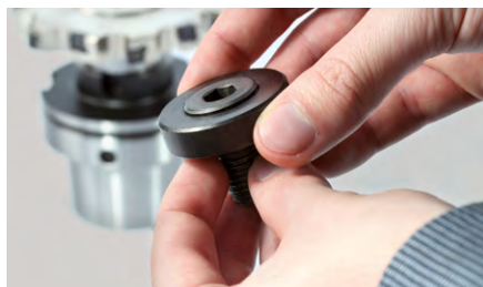
6. Turn threaded bolt until it protrudes 1-2 mm in relation to the threaded ring.
