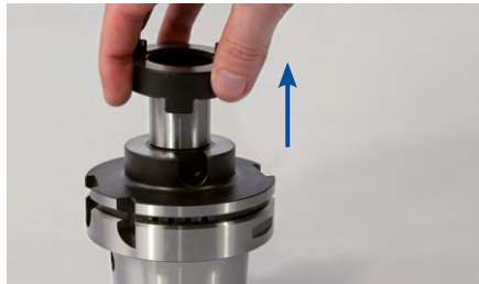
1. Remove the driving ring from the milling cutter arbor.
