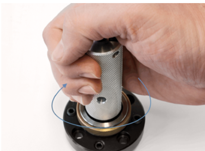
Locking the KS clamping cartridge
