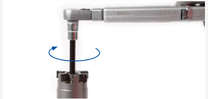
5. Adjust a torque wrench to the tightening torque required by the milling cutter manufacturer.
