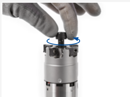
2. Unscrew the milling cutter clamping screw from the thread bore and remove it.
