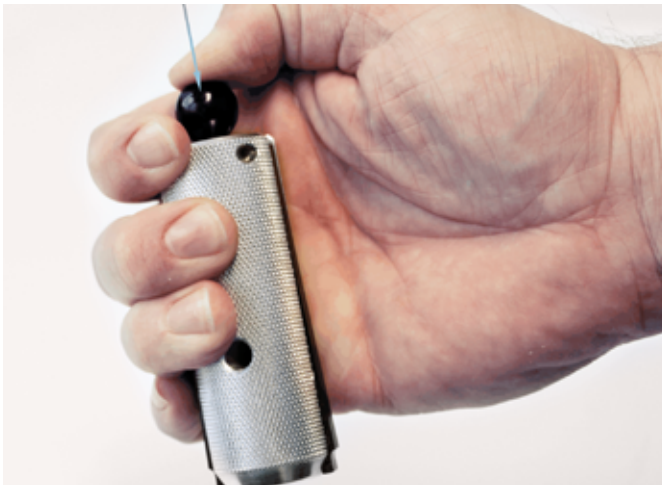
Opening the KS assembly tool
