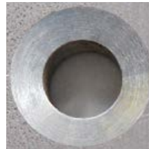
Countersink with extremely unequal spacing
