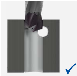
Bore eccentric; chisel edge cutting
