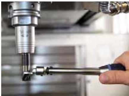
4. As far as is possible, keep the torque wrench horizontal when placing it on the replaceable drill head, thus ensuring the spanner is not tilted relative to the surface.
