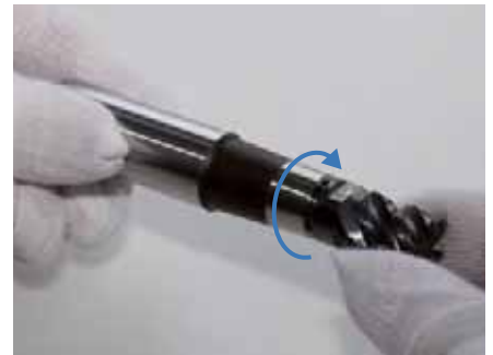
3. Screw the replaceable milling head into the replaceable head holder, turning it tightly by hand. Then, screw the replaceable head holder, along with the tool, into the machine holder.
