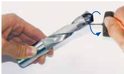
2. Unscrew the clamping screw using the hexagon key supplied.
