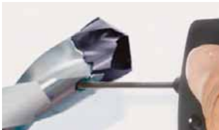
1. Each time you change the drill head, check that the clamping screw is tight. If the clamping screw can be easily loosened, it must be replaced. Only use the original clamping screws!
