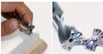
1. Clean the TTS connection of the holder with a brush.
