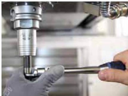
5. Note: Place your free hand on the replaceable milling head so that you are able to carry out delicate tuning. In this way, more precise adjustments can be made to the tightening torque.
