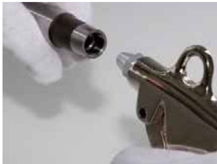
2. Clean the taper, thread and face surface of the replaceable head holder using compressed air and a towel.
