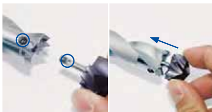
2. Fit the new drill head to the holder.
