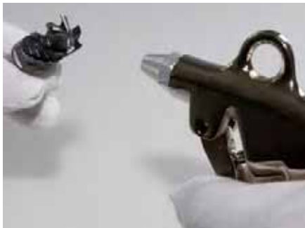
1. Clean the taper, thread and face surface of the replaceable milling head using compressed air and a towel.
