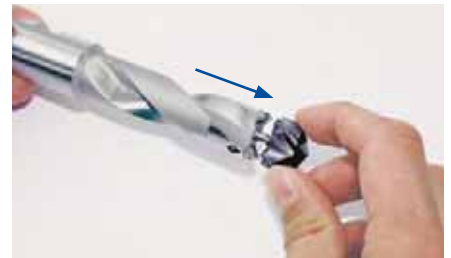
3. Pull the drill head out of the serration.
